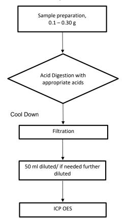
Process Flow for analysis of metal contents in plastics, metals and electronic components sample
