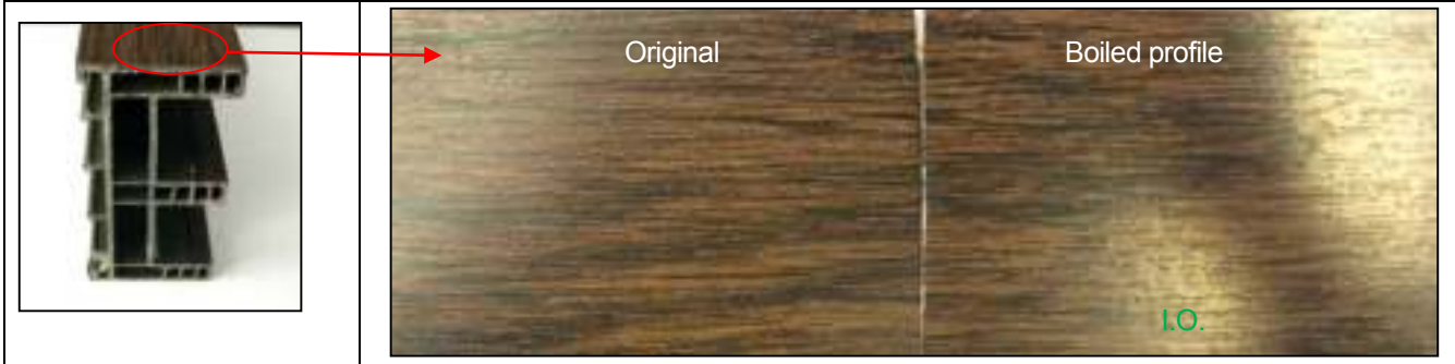
Picture 1 – Boil test according to AMMA 303-18 – Comparison (Original – Boiled profile)
