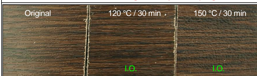
Picture 2 - Bottom side – Heat storage – Comparison (Original – 120°C / 30 minutes – 150°C / 30 minutes)
