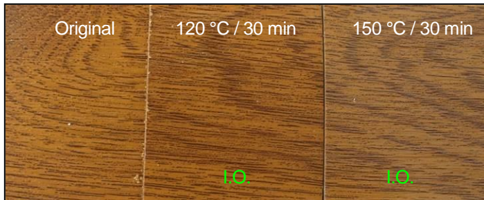
Picture 1 - Upper side – Heat storage – Comparison (Original – 120°C / 30 minutes – 150°C / 30 minutes)
