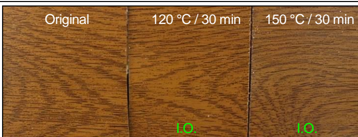
Picture 2 - Bottom side – Heat storage – Comparison (Original – 120°C / 30 minutes – 150°C / 30 minutes)
