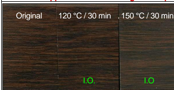
Picture 1 - Upper side – Heat storage – Comparison (Original – 120°C / 30 minutes – 150°C / 30 minutes)
